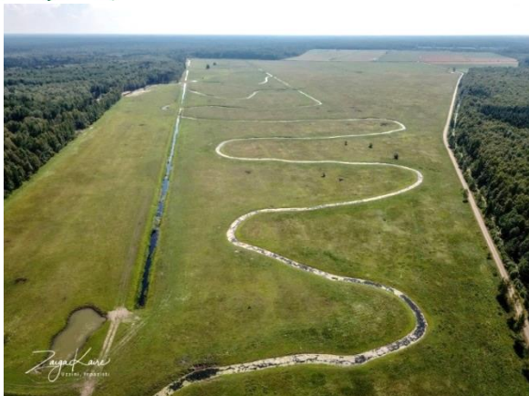
The old (straight) and re-meandered Slampe River, the fenced pasture. The river was restored in 2005 by excavating a new riverbed and blocking the old ditch. The flooding regime is restored; still, the water and ecological quality of the river are poor. Photo: Z. Kaire.
